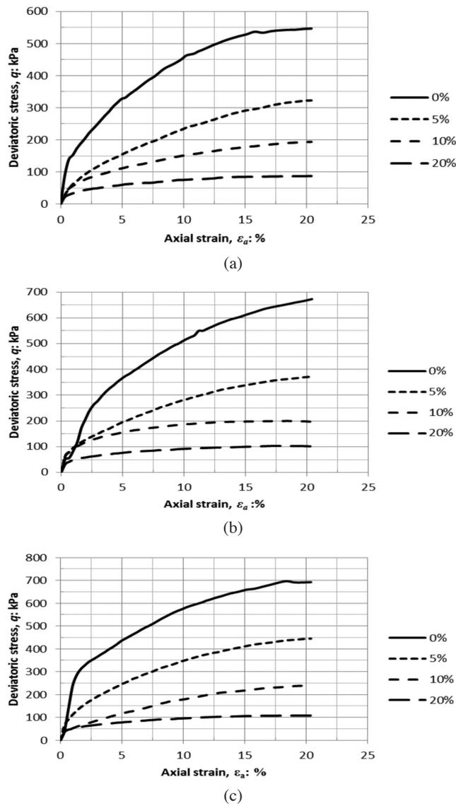
FIGURE 7. Shear-strain of treated soil with surfactant contents at confining stresses of (a) 140kPa, (b) 280kPa and (c) 520kPa
